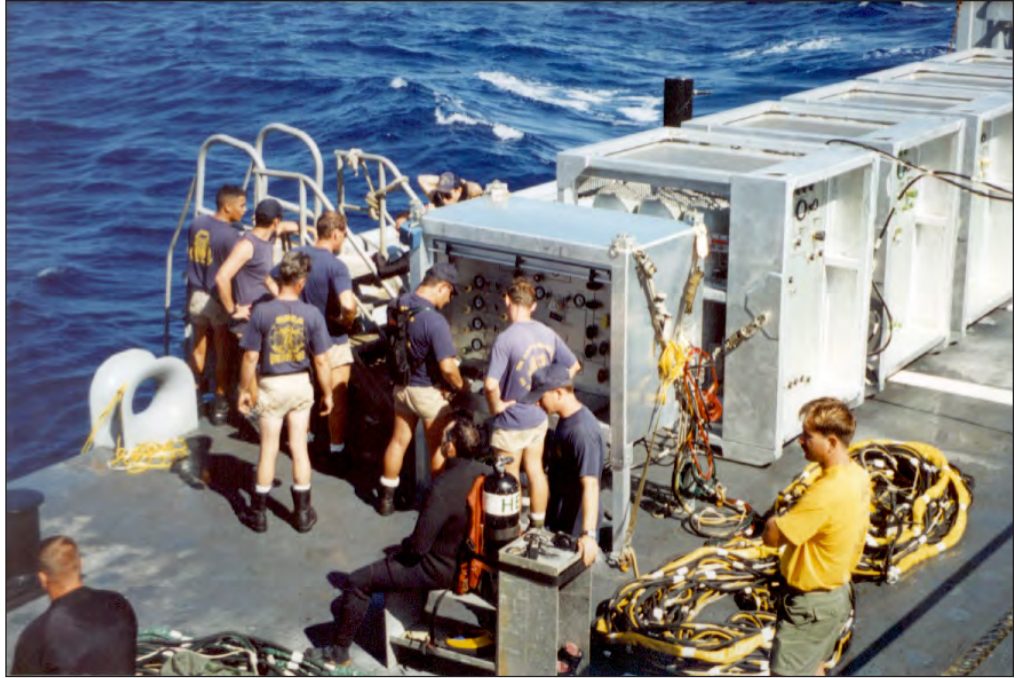
Figure 12-1. FADS III Mixed Gas System (FMGS).
